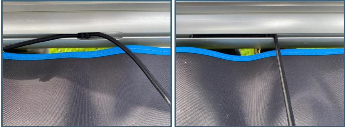
Insert the additional jib track sliders with mounted gennaker blocks, depending on the track end stop you have, you may need to remove the original jib slider first. The gennaker block slider should sit behind the jib cleat slider.
