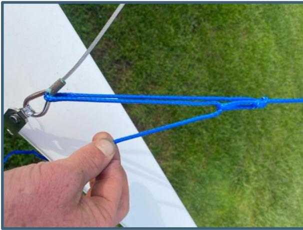
Use the pre-made pole bridal wires to then equally tension the pole to create a small amount of prebend. Use the main bridal eye and the purchase loop to adjust so that the pole remains on the centre line of the boat.
