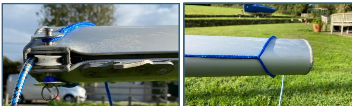
Measure 1750mm down from the mast head, this should be where the halyard block lays. At this level you will need to drill 2 x 5mm holes into the mast track on either side of the section. These need to be 15mm from the trailing edge of the luff groove. This is where the halyard block rail line will attach.
