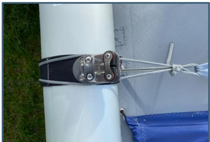
Insert the knot of the provided retrieval bungee (metal ring at other end) into the rear beam track, between the two toe straps. On older boats you may need to remove a hull, but on later boats there is a cut out in the beam slot to make this a simple operation.
